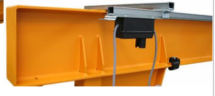
Stationary control on the jib crane (replacement control)
